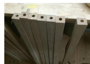
Screw right-handed threaded sleeves into the drill holes. In Switzerland, threaded sleeves are available at Jumbo or in the Hasler Proficenter.
