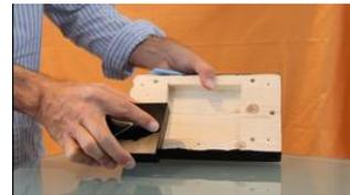
... and then I closed the bottom side with a thin Pavatex board.
