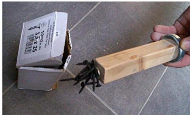
Once the plasterboard is mounted over the steel beam, it is practically impossible to find the metal again and put screws into it. That's where my tool comes in handy! The CSN-48 finds the metal easily and you can just let it hang there upside down. The CSN-16 holds a nice stockpile of screws within reach that you can use to screw the plasterboard onto the steel beam.
