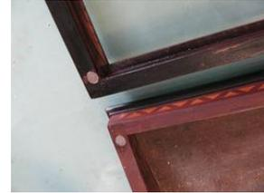
In this case of a table display case, four holes were drilled into the frame of the lid and the case respectively and a total of 8 S-10-01-N ([www.supermagnete.fr/eng/S-10-01-N](http://www.supermagnete.fr/eng/S-10-01-N)) were embedded. These eight magnets help close the display case flush.
