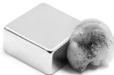
Clean removal: all filings are now embedded in the wax and the magnet is clean again
